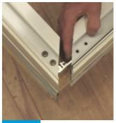
Slide the ringbeam bracket into the channel on the adjoining ringbeam and push together. Fix the ringbeam screws into predrilled holes.
