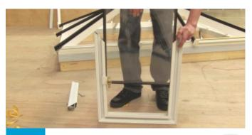
Slide glazing into roof vent sash and press down.
